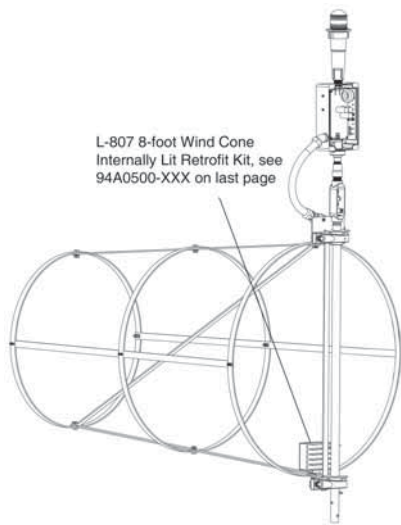
8-foot internally lit wind cone has one LED assembly
