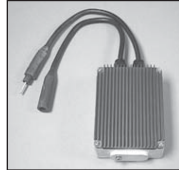
Field Lightning Arrestor
